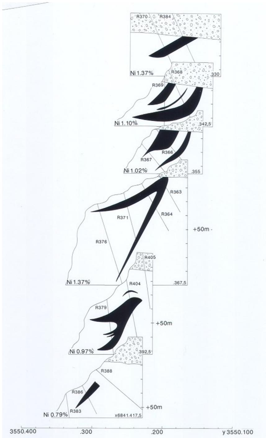
Ore sections (cut off 0.40 % Ni) in the Niinimäki surface ore. View from north to south. Average Ni content marked on each section. From Makkonen & Forss (1994).
