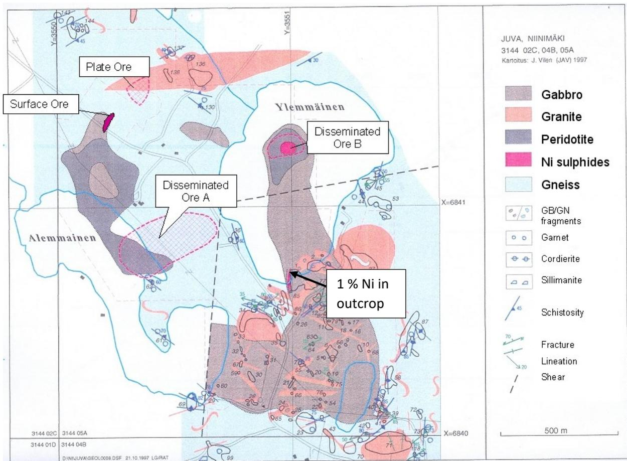
Figure 1. Surface bedrock map of the Niinimäki intrusion and related Ni-Cu-Co deposits and showings, figure modified from GTK website: [http://tupa.gtk.fi/karttasovellus/mdae/raportti/46\\_Niinimäki.pdf](http://tupa.gtk.fi/karttasovellus/mdae/raportti/46_Niinimäki.pdf)
