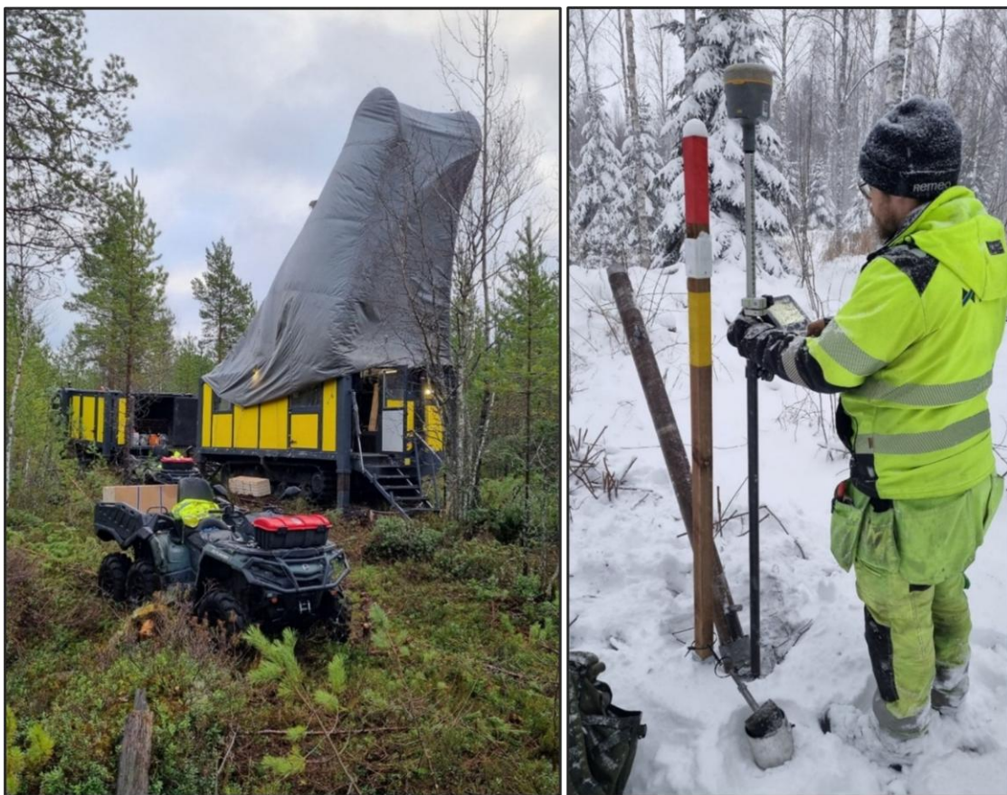
Figure 7-18. Comadev drill rig and ATV at work (left). Mitta Oy surveyor Harri Kujala measuring collar of hole KUP-007 (right). The hole has modified drill rod inserted.
