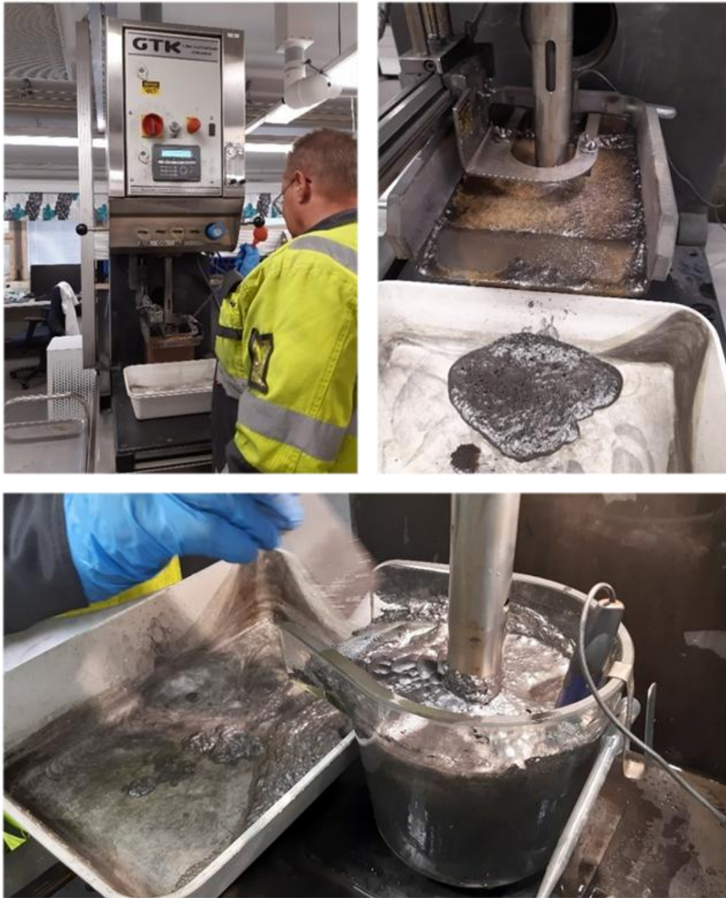
Figure 7-7. Outotec GTK flotation machine (upper left), 4 L flotation cell with automatic froth scrapers (upper right) and a 1.5 L flotation cell with manual froth scraping (down). From Taskinen (2021).
