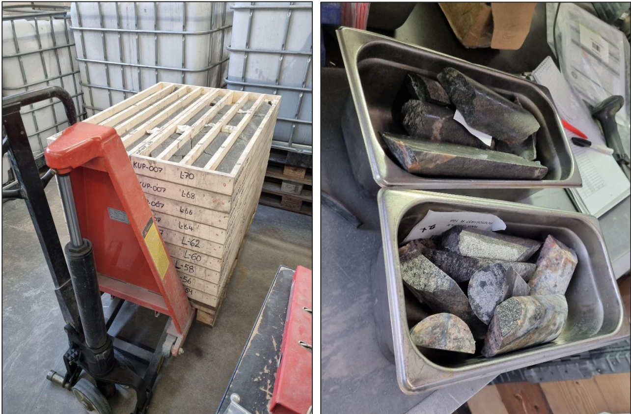
Figure 8-16. On the left, remaining drill core from drillhole KUP-007 after sawing. On the right, weighted samples going for drying in oven. Photos taken at ALS Sodankylä facilities on audition visit, April 2024.
