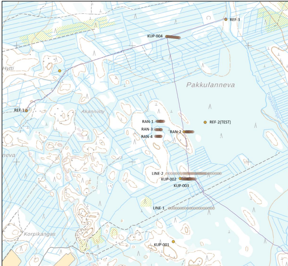
Figure 7-17. Surveyed drill holes and ground lines. REF-1-3 are remote electrode positions tested and used. The remote current electrode was 2.2 km southeast of the survey area, not shown on the map. Modified from Kivinen (2025).
