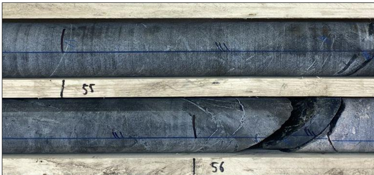
Figure 8-7. Some microfracturing in amphibolite (light veinlets). Hole KUP-007.
