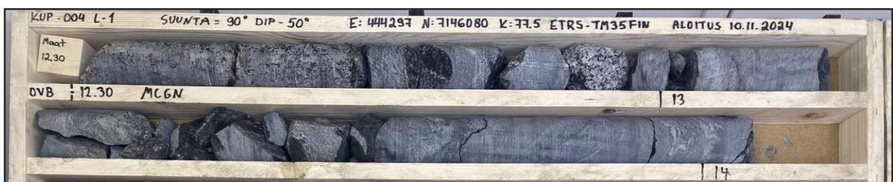
Figure 7-19. First box (=core tray) contains hole number, box number, azimuth, dip, easting, northing, elevation, coordinate system, starting date and overburden thickness.
