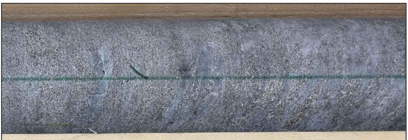
Figure 6-15. Disseminated ore in drill core. Graphite flakes are best seen on the right.
