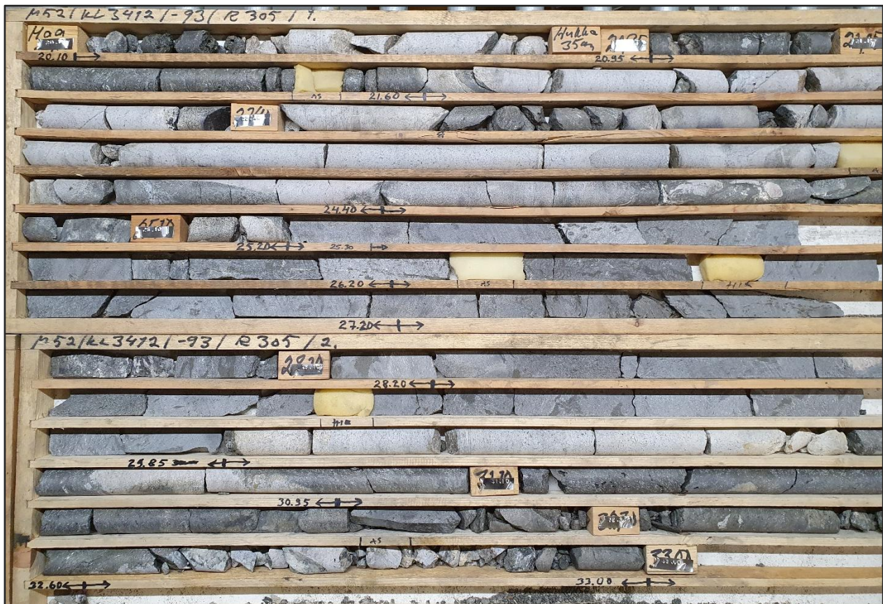
Figure 7-5. Graphite gneiss (dark) and granite (light) in the GTK R305 drill core. Assay intervals of Suomen Malmitutkimus Oy assaying marked.
